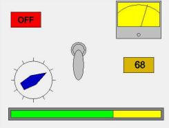
The toggle switch position is changed by rotating the "toggle" handle around the center of the switch. The meter position is changed by rotating the line representing the needle. The progress bar is changed by changing the right side of the green rectangle. The rotary switch is changed by rotating the polygon. The axes and grid lines were suppressed since they did not contribute to the display.
