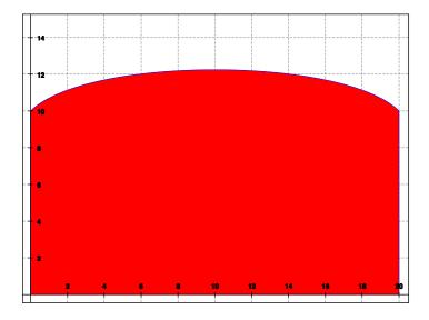
The "complex" shape has a line on the left side, a Bezier curve on the top, and a polyline completing the right and bottom sides. The interior is filled with red, although it could have been filled with any color or hatch pattern.
