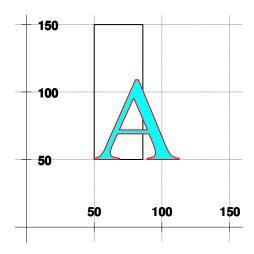
The bottom of the rectangle defines the baseline upon which the character(s) will sit. The left side defines the start point (usually the left edge) of the character(s). The height of the rectangle determines the size, including the descenders (so it appears taller than the character), and the width determines the <u>average</u> character width.
